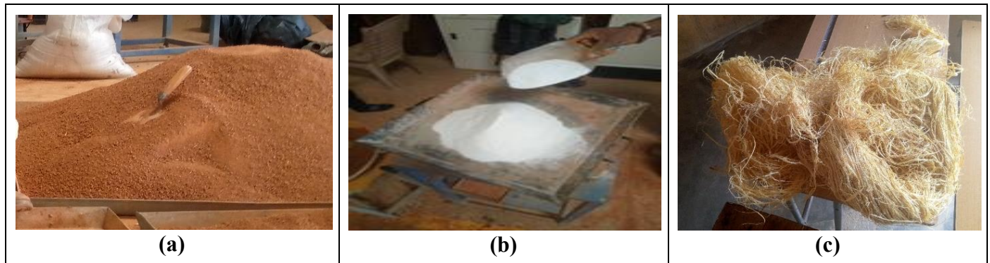
Fig. 1: (a) Earth (b) Milled Glass (c) Cissus Producta Fibre
